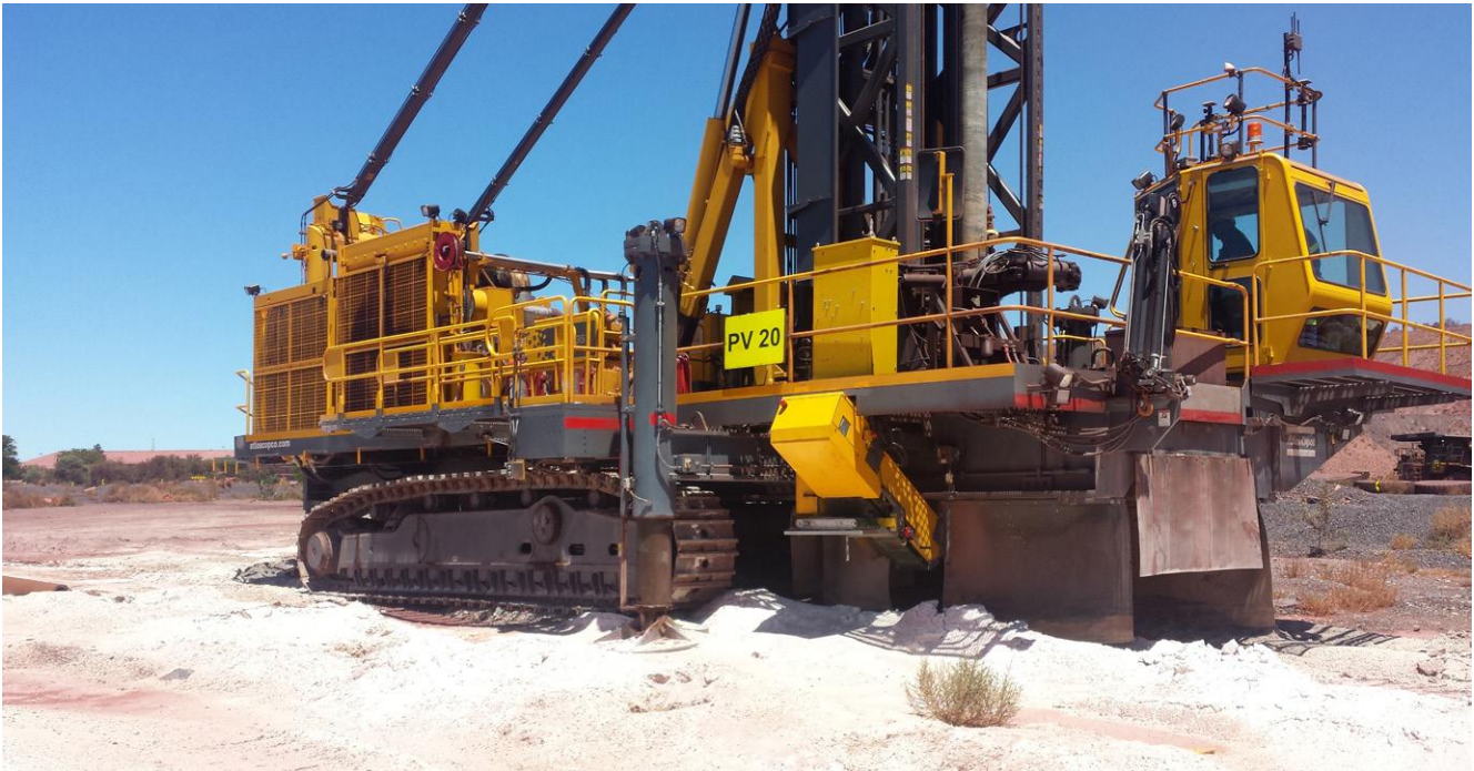
IMA Bulk Ore Sorting System separating ore and waste rock
