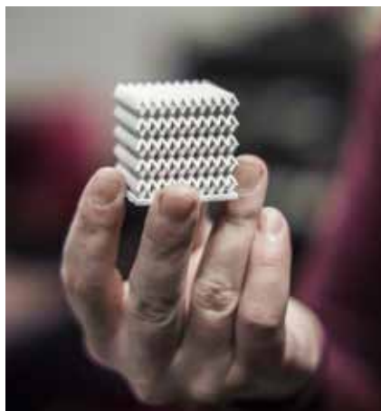
Figure 1. A 3D-printed cell structure using Ceramic Vat Photopolymerization (VPP) technique. Picture by Jonne Renvall/ Ceramic Materials research group/Tampere University.
