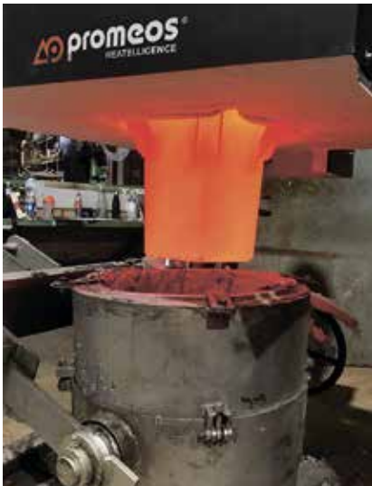
Fig. 1: promeos® ladle preheating system with porous-media burner panels. The glowing burner surface delivers uniform radiant heat into the ladle interior, ensuring through-thickness thermal soaking of the refractory lining.
