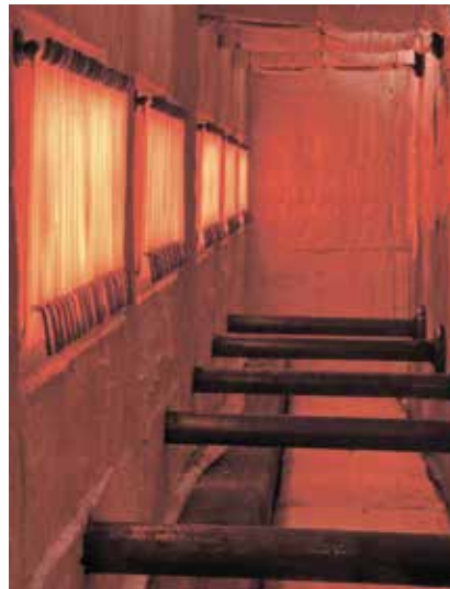
Fig. 2: Close-up of a porous-media combustion burner during operation. The characteristic mesh structure enables flameless oxidation, distributing heat uniformly across the target surface.
